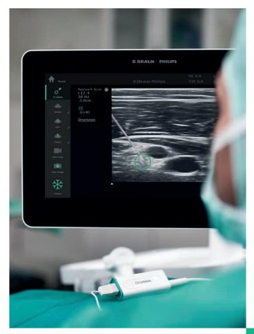
One of the mutual goals of Philips and B. Braun is to make peripheral nerve blocks easier and safer for both healthcare professionals and patients. This goal is now becoming a reality with Onvision<sup>®</sup> – our groundbreaking ultrasound needle guidance system. Tracking the needle tip can be particularly challenging when working with anatomically deep nerves and steep needle angles.
