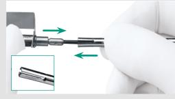
Assemble shaft I Slide the metal inner tube onto the jaw insert with its four spring tongues towards the working end until the tongues snap in place.
