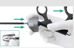
Connect shaft and handle Pull the rotation knob back and hold it. Hold the shaft firmly by its protecting cap and push it into the handle. Release the rotation knob, which moves forward. Important: Do not hold on to the movable handle component.
