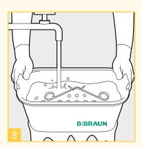
Rinse the instruments thoroughly under cold running tap water.
