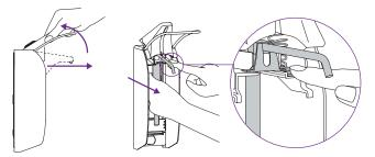
• To insert the pump, slide it in from the front until it engages. Avoid touching the riser pipe. Lower the outlet panel again.
